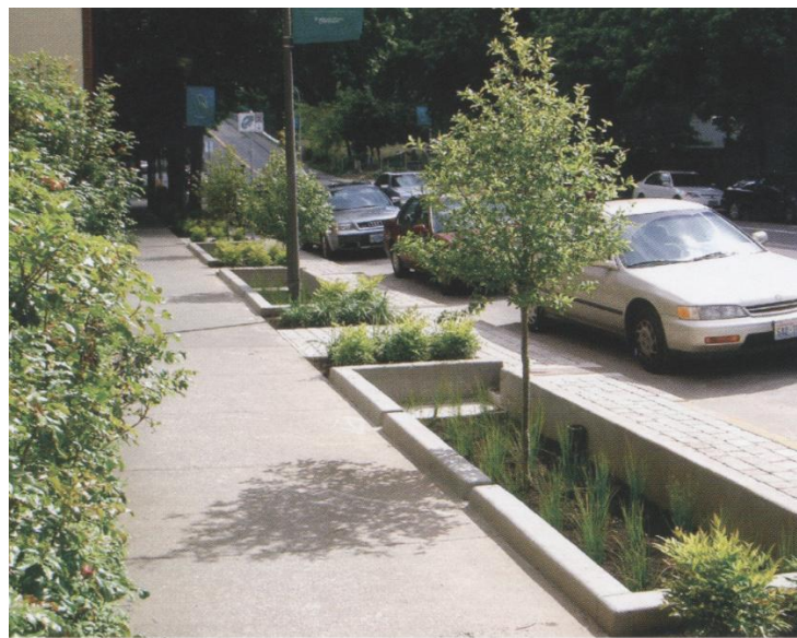
Figure 8: Curbside pond catching sidewalk runoff
